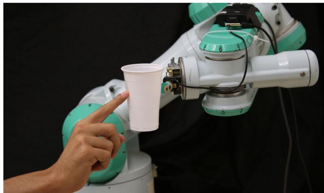
Fig. 1. A human-robot grip stabilization experiment where a human and a robot collaborate in order to preserve a stable grip on a deformable plastic cup. A detailed description of the experiment can be found in Section 3.7. Results show that the robot is able to respond to actions taken by the human in order to keep the object from slipping. The experimental results are discussed in Section 4.6.
